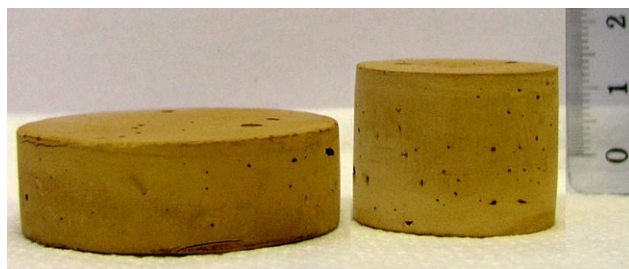
Figure 1. Monoliths obtained from castor oil-in-black liquor emulsions. [Color figure can be viewed in the online issue, which is available at wileyonlinelibrary.com .]
